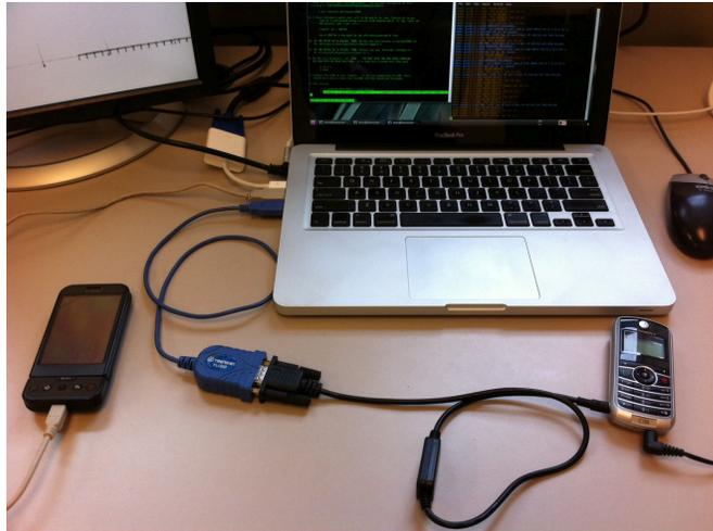
**Figure 3.** Our testbed showing the C118 running the GSM layer 1 (bottom right), the laptop running the GSM layer 2 and 3, and a T-Mobile G1 (bottom left) used as our mapping tool and later our victim.
